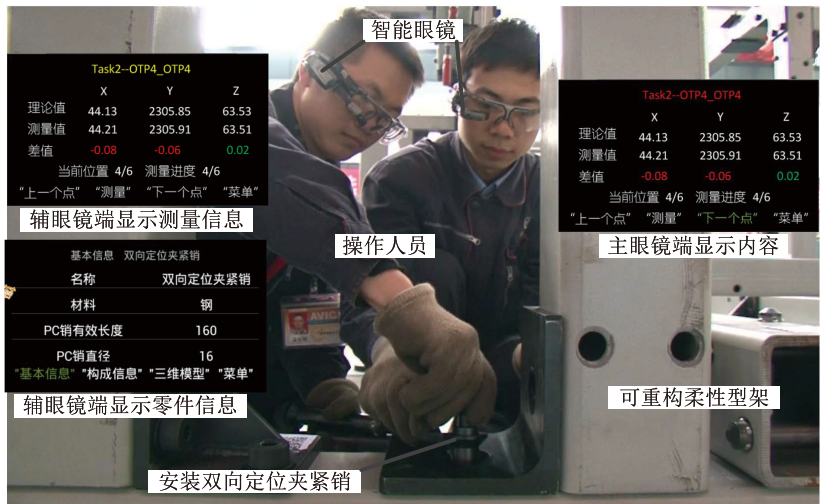
图9 操作人员佩戴智能眼镜装调型架 Fig.9 Operators assemble tooling with smart glasses
